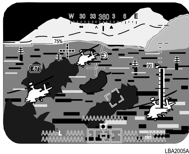
Figure 4-26. FCR Profile Lines and Obstacles in C-Scope
