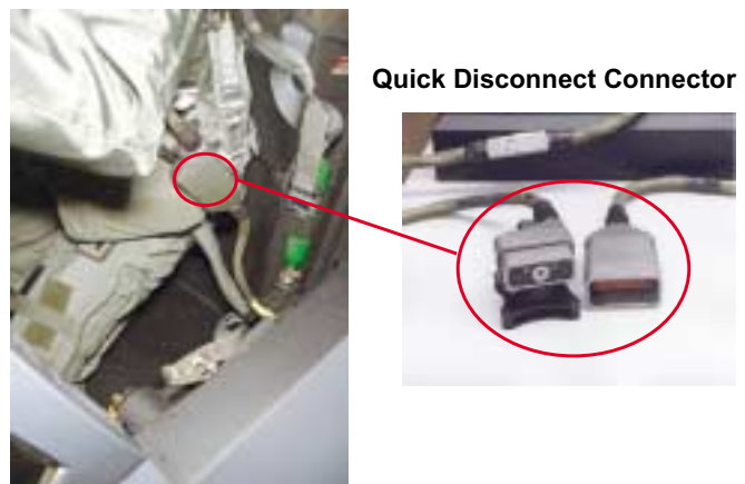
Figure 6-7 Hip Quick Disconnect
