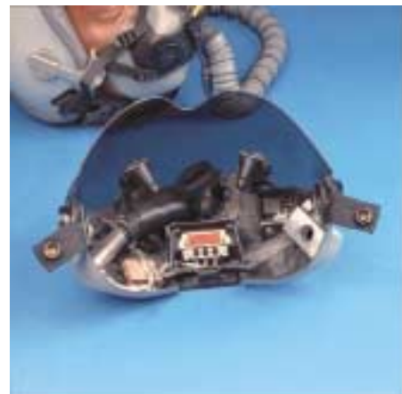
Figure 6-3 Helmet Mounted Display Unit
