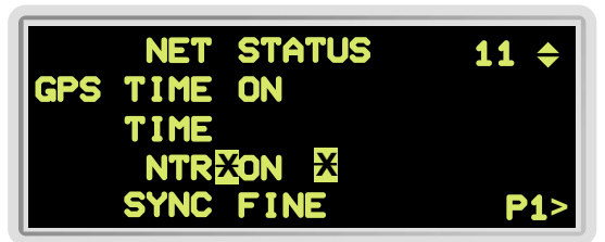
Figure 8-10 NTR Field on the Link 16 Init Page 1
