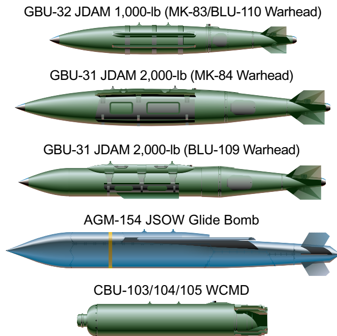
Figure 7-1 Inertially Aided Munitions
