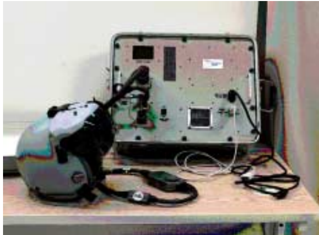
Figure 6-4 HMCS Helmet Test Set
