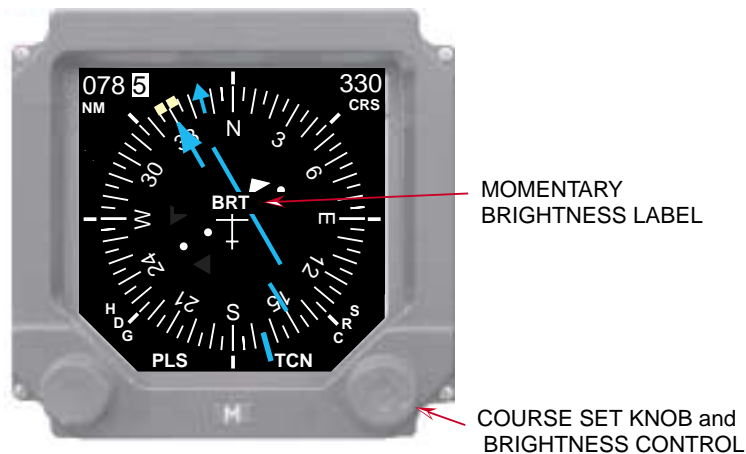
Figure 9-9 EHSI Brightness Adjust
